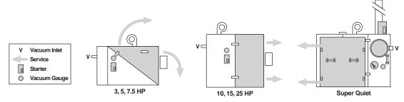
Specifications not listed below are the same as those listed above. All Sound Enclosures include a cooling fan 115 VAC @ 2 amps.
